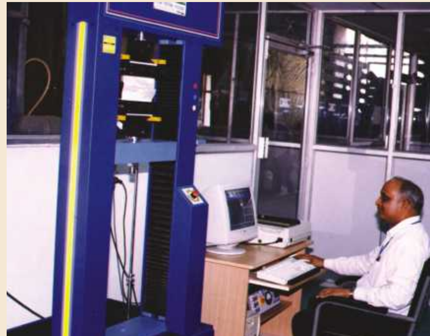
Wide width tensile test in progress
